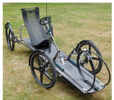
Each pedal engages onto its own belt. This belt is wrapped around the freewheel on the rear wheel axle.
